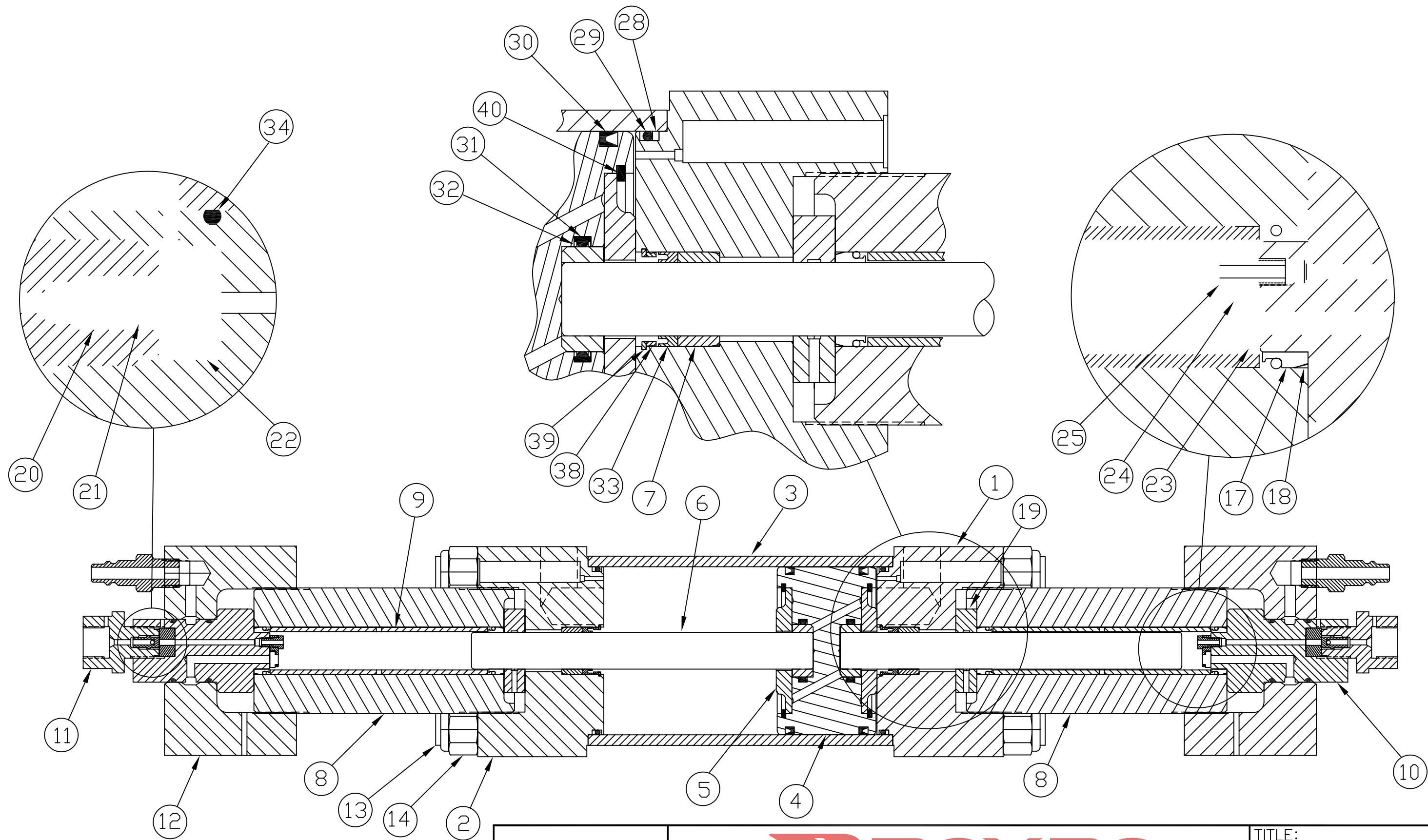
NOTES: USE 4 3/8-16 X 2.5 SHCS TO ATTACH MANIFOLD TO INTENSIFIER.
