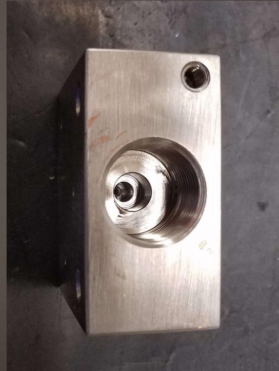
11. Install retaining nut onto new needle and install new needle making sure that is flush on the top.
